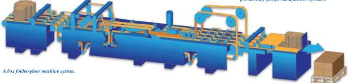
Folder-gluer machines normally use three or more different types of nylon core belts. These include feeder-type belts, folder-gluer belts, and traditional conveyor belts. Each belt is designed for a specific use on the machine and made to handle either light, medium, or heavy shock loads.
